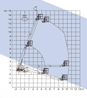
Max platform height: 13 m Max working height: 15 m Max moveable load: 250 kg
